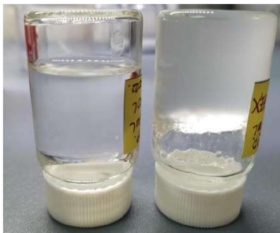
Figure 1 Ethanol (left) and cyclohexanol (right) standard pesticide solution after being stored at low temperature (4°C)
