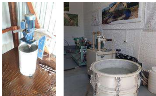
Figure 1 Leaching and filtering of the composite sample of flotation tailings COMPOSITE I+III at the pilot plant
