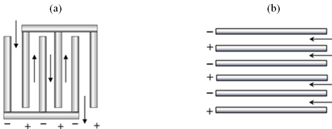
Figure 4 Mode of electrodes construction and water flow: (a) vertical single channel, (b) horizontal multiple channel
