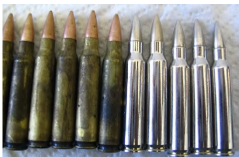
Figure 1. Treated samples with methods with mercury-nitrate solution (right) and ammoniacal copper-sulphate a solution (left)
