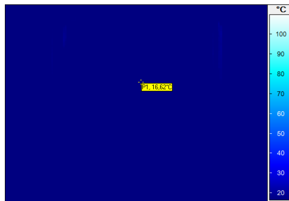
Figure 2. Thermographic display of sample with Lechsys matte coating at room temperature
