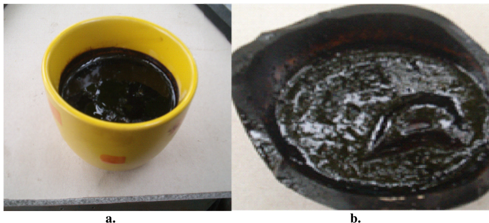
Figure 5. Sample of soil soaked with oil before (a) and after the treatment (b)
