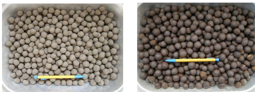
Figure 7. View of M4 raw granulates and their expansion product at 1110 °C for 15 min.
