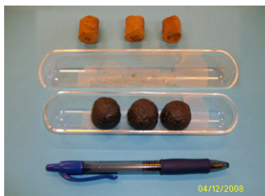
Figure 2. General view of raw granulates M2 and after expansion at 1150 °C for 15 min.
